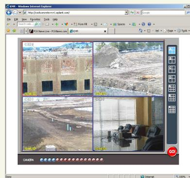
Traveling to and from job sites to monitor progress or solve problems is time consuming and costly. A high-res remote controlled Internet camera allows supervisors and key personnel to view your jobsite from any computer with web access.
